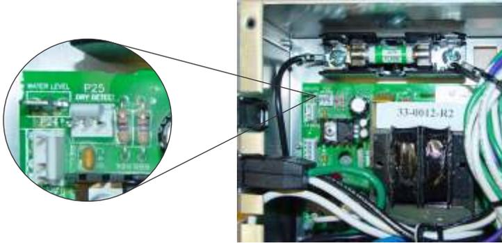
1. Locate the connection point for the flow switch.
