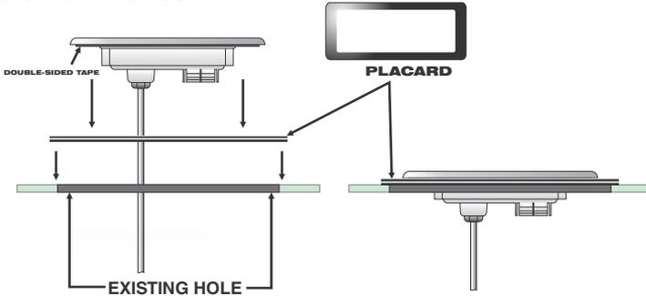
**Step 3** – Remove protective film from display windows, clean control surface with rubbing alcohol and apply label. Connect spaside control plug to circuit board as shown.
