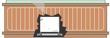
Power from main breaker panel to service disconnect within line-of-site of the spa to portable spa control equipped with built-in GFCI.
