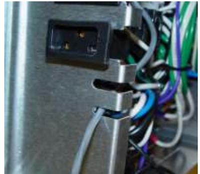
3. Route the flow switch cable through an empty slot allocated for small cables/cords.
