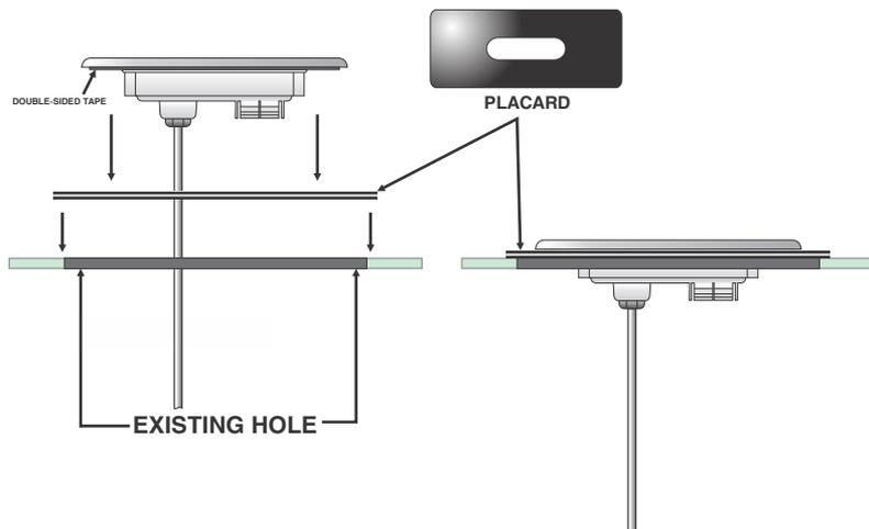
**Step 1** - (If control cutout already exists, determine if placard must be used. If existing cutout is sufficient, disregard step 1.) **Choose a location for the spaside control. Using the template provided, drill two 1" diameter holes, 2 5/8" apart. Cut away the material between the two holes, clean area and insert spaside.** (If placard is required, position and secure using a water resistant silicone sealant.)
