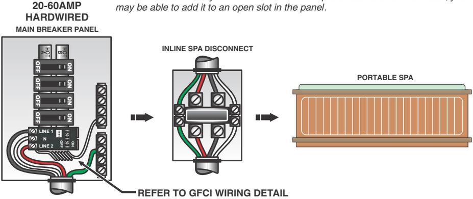
*Power from GFCI breaker installed into main service panel to a service disconnect within line-of-site of the spa.*
