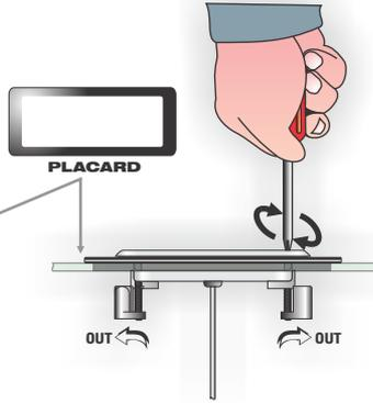
**Step 1** – (If control cutout already exists, determine if placard must be used. If existing cutout is sufficient, disregard step 1.) **Choose a location for the spaside control. Using the template provided, cut out a 2 5/8" X 6 3/8" hole. Clean area and insert spaside control making sure tab locks are rotated inward.** (If placard is required, position and secure using a water resistant silicone sealant.)
