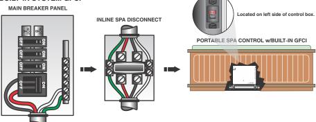
Power from main breaker panel to service disconnect within line-of-site of the spa to portable spa control equipped with buit-in GFCI.
