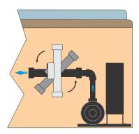
The heater can be installed vertical, horizontal or at an angle in the pumps discharge plumbing (providing position DOES NOT allow air pockets to form inside the housing). The heater can be installed up to 5-feet from the control system, which is connected via a black 3-conductor and black 6-conductor cord to the black receptacles
