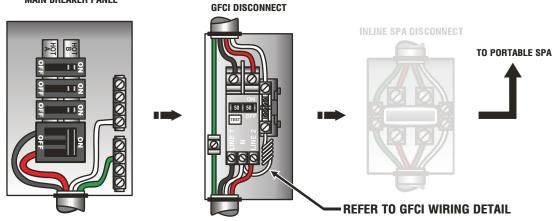
Power from main service panel to a GFCI subpanel within line-of-site of the spa. (Note: Most local codes will allow a GFCI subpanel to be a disconnect. If this is not the case in your installation, a disconnect must be provided.)
