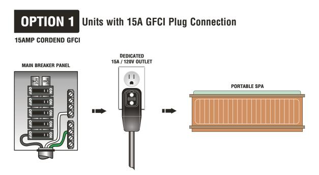
This illustration depicts a typical 15 AMP, cord-end GFCI installation. (The spa must be installed on a dedicated circuit.)
