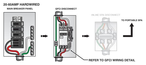
Power from main service panel to a GFCI subpanel within line-of-site of the spa. (Note: Most local codes will allow a GFCI subpanel to be a disconnect. If this is not the case in your installation, a disconnect must be provided.)
