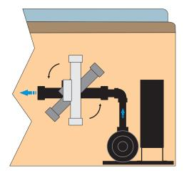
The heater can be installed vertical, horizontal or at an angle in the pumps discharge plumbing (providing position DOES NOT all air pockets to form inside the housing). The heater can be installed up to 5-feet from the control system, which is connected via a black 3-conductor and black 6-conductor cord to the black receptacles provided at the control box..
