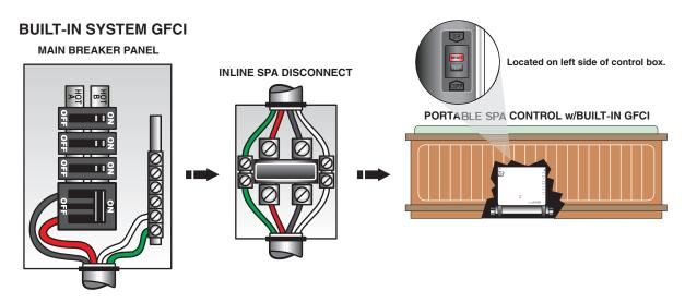
Power from main breaker panel to service disconnect within line-of-site of the spa to portable spa control equipped with buit-in GFCI.
