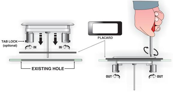
Step 1 - (If control cutout already exists, determine if placard must be used. If existing cutout is sufficient, disregard step 1.) Choose a location for the spaside control. Using the template provided, cut out a 2 5/8" X 6 3/8" hole. Clean area and insert spaside control making sure tab locks are rotated inward. (If placard is required, position and secure using a water resistant silicone sealant.)
