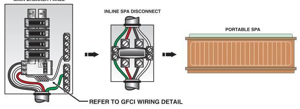
Power from GFCI breaker installed into main service panel to a service disconnect within line-of-site of the spa.
