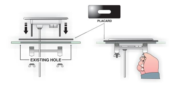
Step 1 - (If control cutout already exists, determine if placard must be used. If existing cutout is sufficient, disregard step 1.) Choose a location for the spaside control. Using the template provided, drill two 1" diameter holes, 2 5/8" apart. Cut away the material between the two holes, clean area and insert spaside. (If placard is required, position and secure using a water resistant silicone sealant.)
