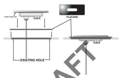
Step 1 - (If control cutout already exists, determine if placard must be used. If existing cutout is sufficient, disregard step 1.) Choose a location for the spaside control. Using the template provided, drill two 1" diameter holes, 2 5/8" apart. Cut away the material between the two holes, clean area and insert spaside. (If placard is required, position and secure using a watervesistant silicone sealant.)
