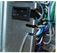
3. Route the flow switch cable through an empty slot allocated for small cables/cords.
