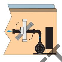
The heater can be installed vertical, horizontal or at an angle in the pumps discharge plumbing (providing position DOES NOT allow air pockets to form inside the housing). The heater can be installed up to 5-feet from the control system, which is connected via a black 3-conductor and black 6-conductor cord to the black receptacles provided at the control box..
