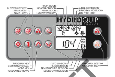
**Default System Operation:** When power is applied, or there is a temporary loss of power, the system will initiate its default programming. The filter cycle will begin 24-hours after the system has been powered up. The filtration cycle will be active for 1-hour and will repeat every 24-hours. The temperature will be maintained at 95BF.
