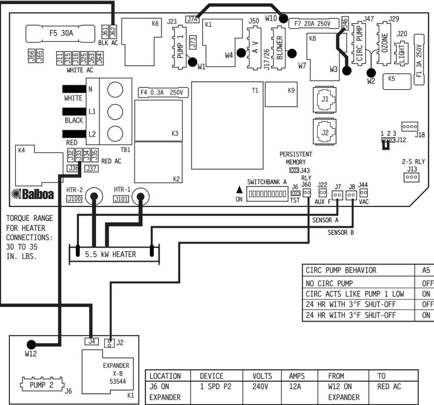
USE COPPER CONDUCTORS ONLY. EMPLOYER UNIQUEMENT DES CONDUCTEURS DE CUIVRE. #6 AWG MIN. WIRE= 90°
