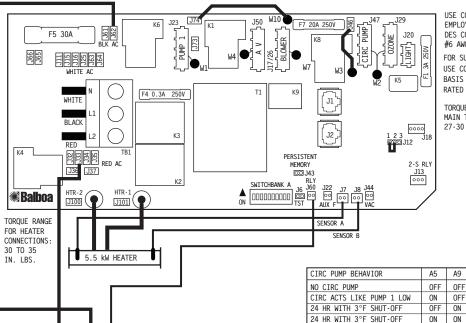
USE COPPER CONDUCTORS ONLY. EMPLOYER UNIQUEMENT DES CONDUCTEURS DE CUIVRE. #6 AWG MIN. WIRE= 90°
