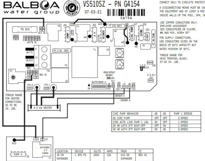
CONNECT ONLY TO CIRCUITS PROTECTED BY A CLASS A GFCI.
