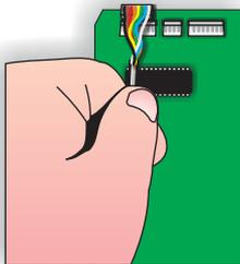
**Step 3** - Remove protective film from display windows, clean control surface with rubbing alcohol and apply label. Connect spaside control plug to circuit board as shown.
