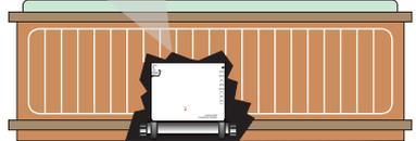
Power from main breaker panel to service disconnect within line-of-site of the spa to portable spa control equipped with built-in GFCI.
