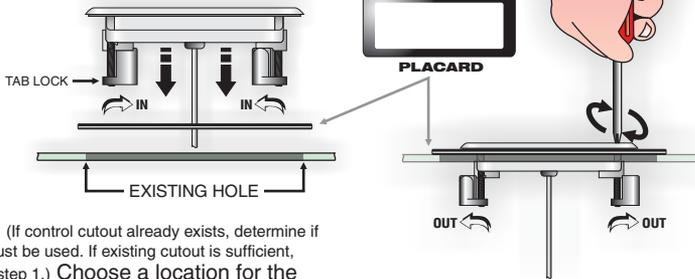
**Step 1** - (If control cutout already exists, determine if placard must be used. If existing cutout is sufficient, disregard step 1.) Choose a location for the spaside control. Using the template provided, cut out a 2 5/8" X 6 3/8" hole. Clean area and insert spaside control making sure tab locks are rotated inward. (If placard is required, position and secure using a water resistant silicone sealant.)
