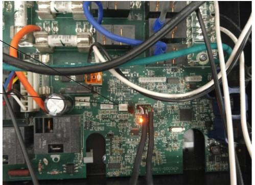
1. Locate the connection point for the flow switch.
