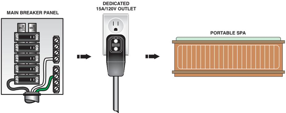
This illustration depicts a typical 20 AMP, cord-end GFCI installation. (The spa must be installed on a dedicated circuit.)
