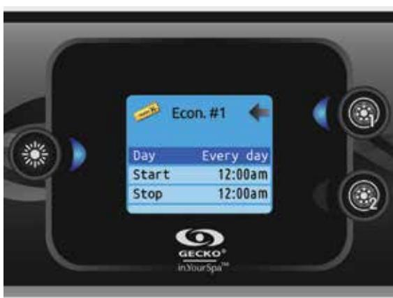
The filtration schedule shown on the screen will apply to the main filtration pump, most likely pump 1. If your spa uses a circulation pump configured to run 24 hours, the screen will show you the purge setting instead of filtration. The purges are pre-programmed for a fixed number of minutes, therefore the duration will be set to N/A on the screen, and only the start time can be modified.
