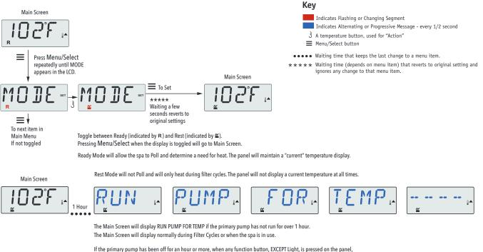
If the primary pump has been off for an hour or more, when any function button, EXCEPI Light, is pressed on the pane the pump used in conjuncton with the heater will run so that temperature can be sensed and displayed.
