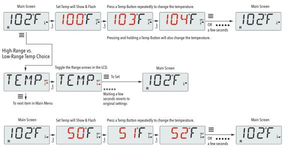
Pressing and holding a Temp Button will also change the temperature.
