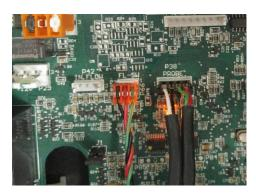
2. Connect the flow switch connector to the connection point (P66) making sure all pins are covered.
