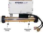
If you need to utilize the slide brackets simply remove the (2) 3/8" nuts securing the heater to the foot brackets and remove from under the box.
